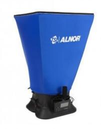
The Alnor EBT731 Balometer Capture Hood is a multipurpose electronic air balancing instrument primarily used for efficiently taking direct air volume readings at diffusers and grilles. The EBT features a detachable micromanometer which can be used with optional probes for increased flexibility in multiple measurement applications.
